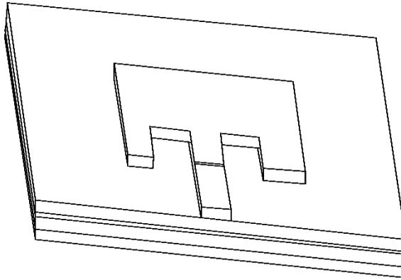
Figure 4. Structure of Wearable HIS Patch Antenna
