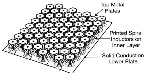
Figure 2. Cross Section View of High Impedance Surface
