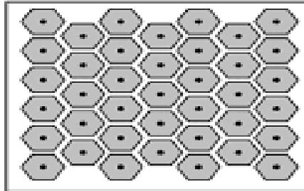
Figure 3. Top View of a High Impedance Surface
