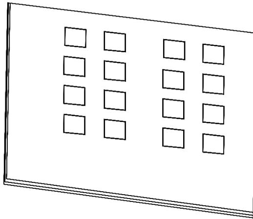
Figure 6. High Impedance Surface
